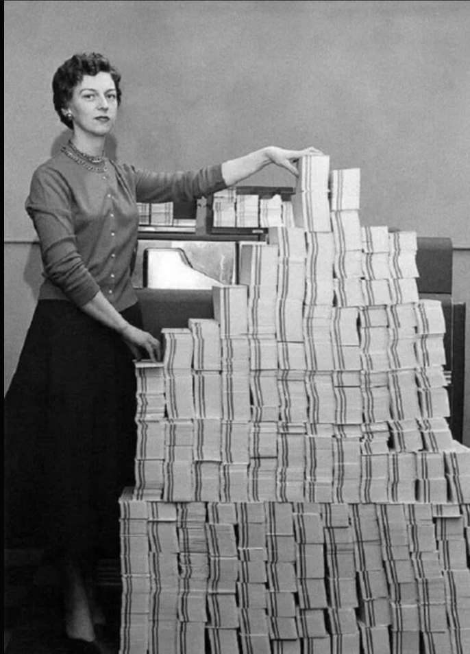
4.5 megabytes of data in 62,500 punched cards, USA, 1955
